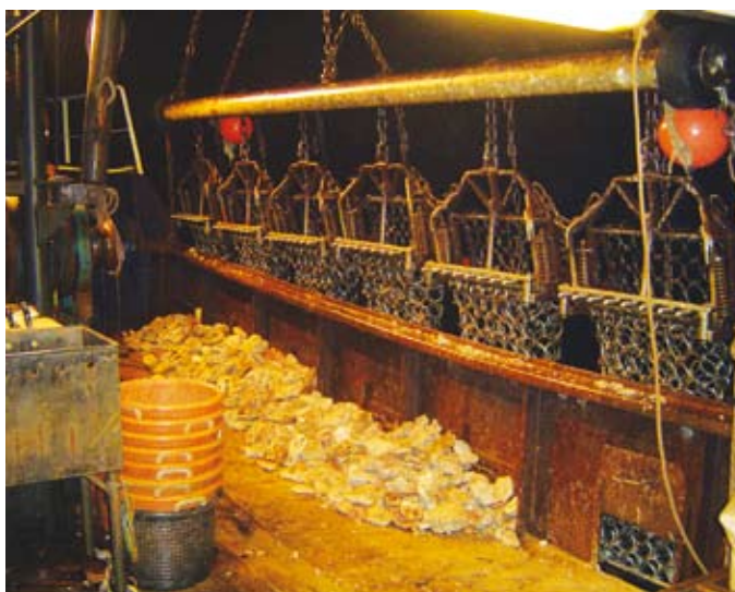
Fig 2. Scallop dredges hanging over the gantry of a fishing vessel and the catch on deck © Sussex IFCA
