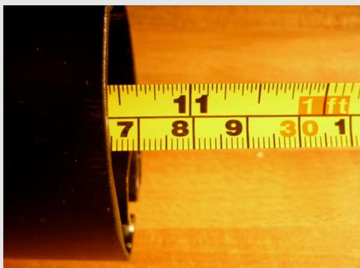
Slide the insert into the mast until the top edge is 265mm below the top of the lower mast section (Photo 3).
