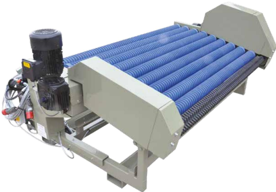
The new Coil Cleaner Plus spiral cleaner moves the crop continuously, separating loose soil, clods and small potatoes from the main crop.
