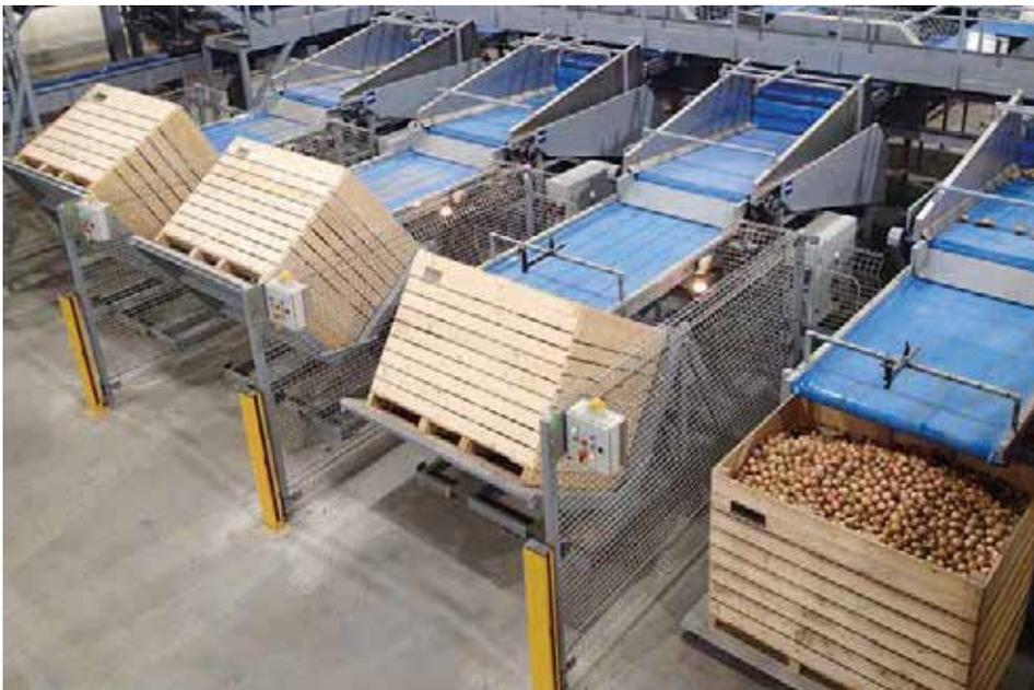
The Herbert single box filler provides gentle and efficient box filling from grading and packing lines by lifting the box to almost a 90 degree angle. Produce is delivered onto the side of the box, keeping the transfer height to a minimum. Under probe control the box then lowers as its fills until its fully down position is reached. The final signal indicates the box is full and if required stops the equipment feeding the system.
