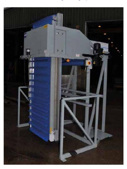
This versatile system is used for the very gentle and highly effective crop placement into boxes, tonne bags and bulk cartons. The produce is carried in pockets vertically down into the receiving container and is released at the last opportunity under probe control.
