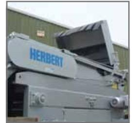
The GF2 Twin Gentle Box Filler gives efficient handling and low drop delivery of crop into boxes preventing damage
