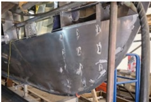
April to August 2024 hull plating
