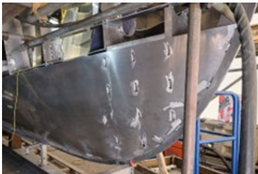
April to August 2024 hull plating
