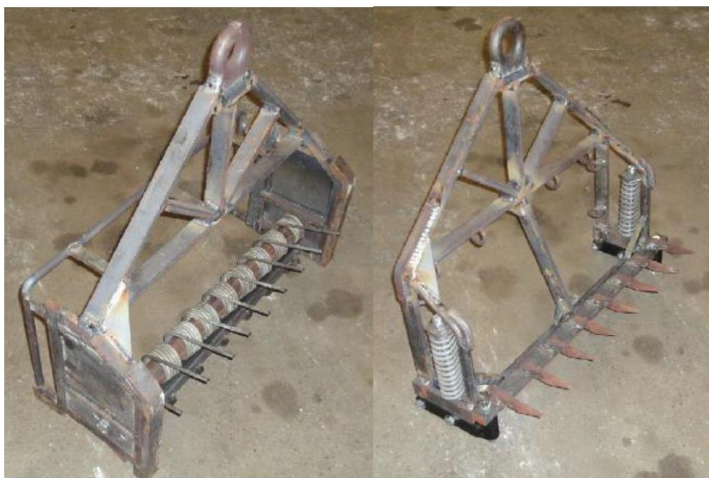
Figure 3. N-Virodredge design (left) separate from the steel belly bag, with individually sprung tines and side skirts; compared to the Newhaven dredge (right) with a fixed tooth bar. Source: Filippi, 2013.
