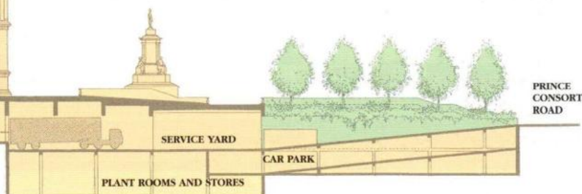
Below: The Royal Albert Hall: section through the rebuilt south steps and service yard.
