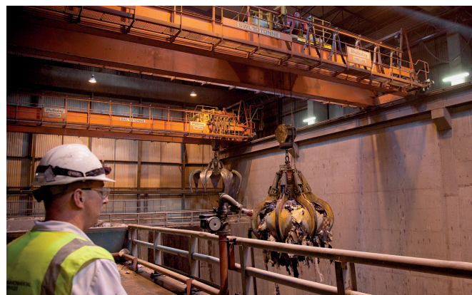
Simon Birkett watching the 'grab' shifting 5 tons of waste at a time
