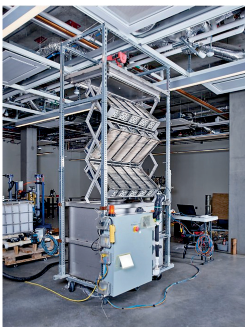
A mechanical tree which sucks carbon dioxide out of the air like its natural counterpart and then stores it safely
