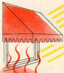
CANVAS AWNING —aluminum painted—22% of Sun Ray heat enters room—light and visibility much reduced—78% efficiency.
