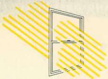
UNSHADED WINDOW —100% of direct Sun Ray Heat enters window—Complete visibility, but zero heat stopping efficiency.
