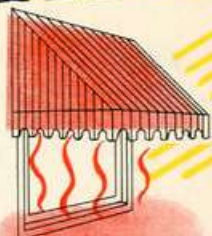
CANVAS AWNING —plain—28% of Sun Ray heat enters room—light and visibility much reduced—72% efficiency.
