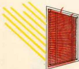
INSIDE VENETIAN BLIND —covering full window—slats at 45°—58% of Sun Ray heat enters window—Almost no visibility.
