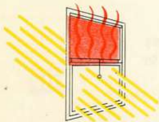
INSIDE SHADE —buff—half drawn—68% of Sun Ray heat enters room. Reduced visibility, 32% efficiency.
