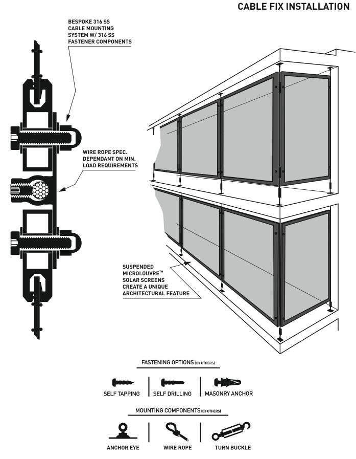
ALL EXTRUSIONS ARE POLYESTER POWDER COATED IN ANY RAL COLOUR COMMERCIALLY AVAILABLE POWDER COAT TO MEET OR EXCEED ISO 2409 AND ISO 9227. ALL DRAWINGS HERE ARE FOR ILLUSTRATIVE PURPOSES ONLY AND NOT TO SCALE.
