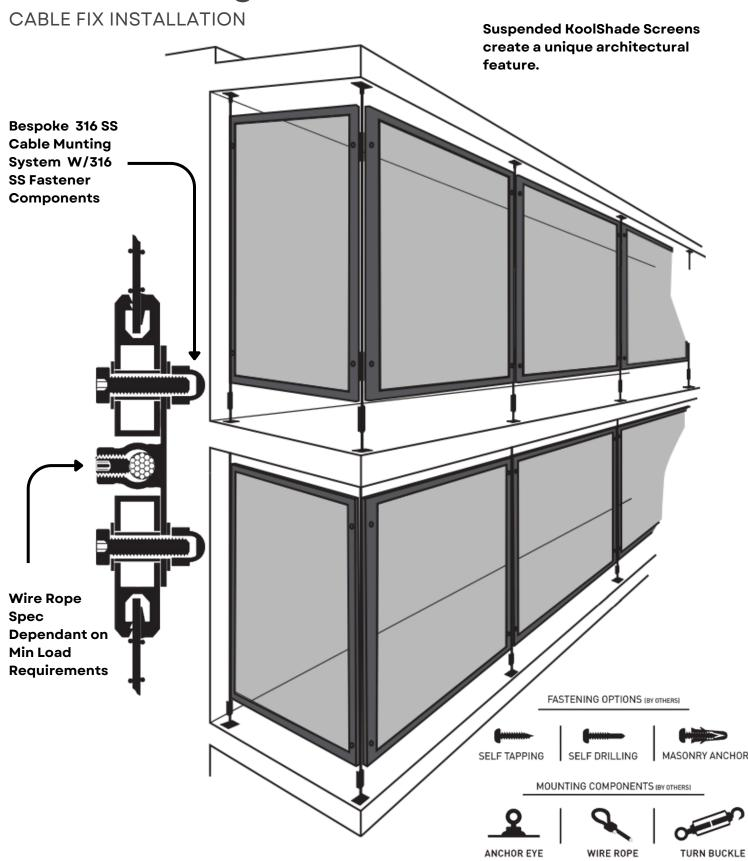
ALL EXTRUSIONS ARE POLYESTER POWDER COATED IN ANY RAL COLOUR COMMERCIALLY AVAILABLE POWDER COAT TO MEET OR EXCEED ISO 2409 AND ISO 9227. ALL DRAWINGS HERE ARE FOR ILLUSTRATIVE PURPOSES ONLY AND NOT TO SCALE.
