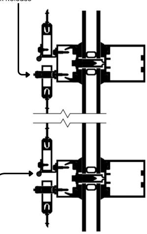
OH78 Offset Hinge Mounting Allows for Easy-Access for Glazing Maintenance
