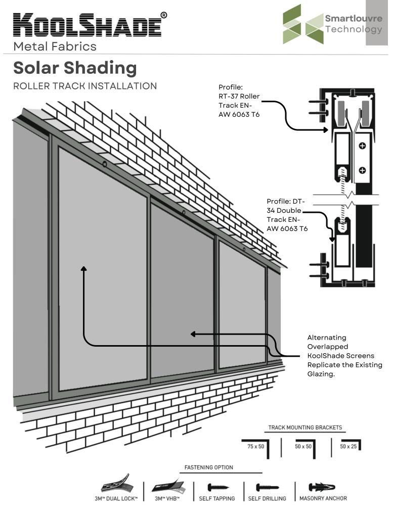
ALL EXTRUSIONS ARE POLYESTER POWDER COATED IN ANY RAL COLOUR COMMERCIALLY AVAILABLE POWDER COAT TO MEET OR EXCEED ISO 2409 AND ISO 9227. ALL DRAWINGS HERE ARE FOR ILLUSTRATIVE PURPOSES ONLY AND NOT TO SCALE.
