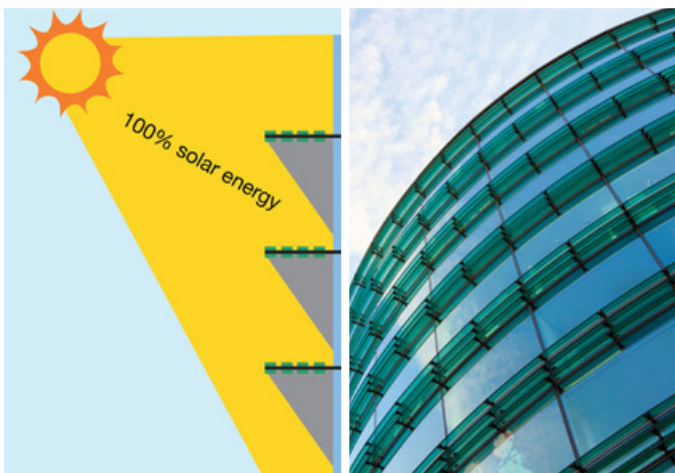
A typical brise soleil system to help reduce solar heat gain and glare by using a horizontal protection from the sun side façade on a building.
