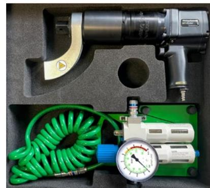
Each kit consists of Pneumatic Torque Wrench, Air Control Unit (NRP-CU), 4m Air Hose (AH4M), Storage Case (2010883), Calibration Certificate, Operating Manual/Parts List
