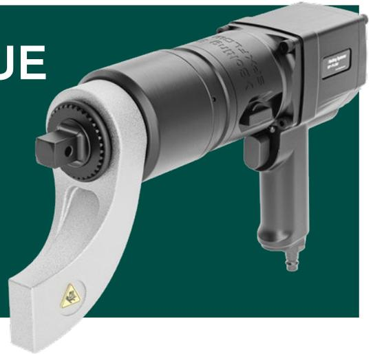
Incorporating a robust planetary gear system driven by a pneumatic motor through a two-speed transmission, our Pneumatic Torque Wrenches offer high speed and accuracy. Each wrench is individually calibrated to establish an accurate relationship between desired torque and corresponding air pressure, resulting in output torque accuracy and repeatability of +/- 3%. Automatic switch-off function at the desired torque aids the user in establishing reliable and repeatable operation.
