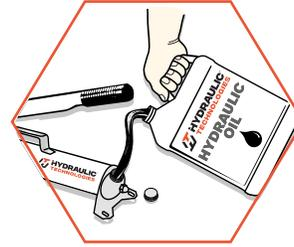
Use only high quality oil, like Hydraulic Technologies hydraulic oil. Using the wrong fluid can lead to equipment damage and premature failure.
