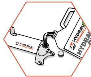
Do not overfill pump reservoirs.
