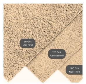
Position your boards on a dry, flat, level surface. Start sanding the boards with an 80 grit sand paper, working with the grain of board and sanding until any debris or pencil marks are removed. Then move to 120 grit and finally 180 grit, brushing off any excess dust or debris prior to oiling.
