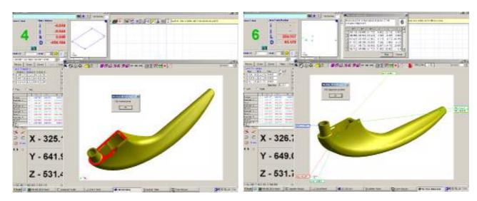
Having aligned to the CAD model, any points taken in any measured feature will now appear in the CAD window. These points will be displayed as a colour-coded dot on the model, and can either have a line leading to a box showing the error of the measured point, or alternatively the length of the attached line can be proportional to the error. In this way it is easy to visualise the distortion of a surface relative to the theoretical model:
