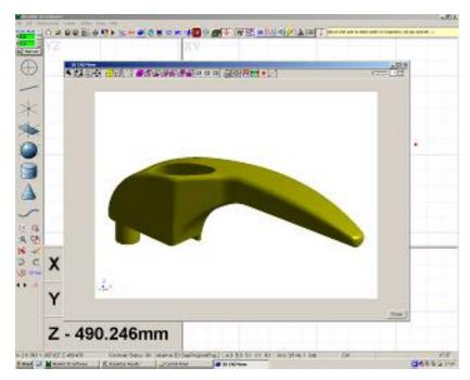
Aberlink's CAD comparison module allows users of the Aberlink 3D software to import a solid model from CAD in either a STEP or an IGES format, and then take measurements using the CAD model as master data. This can be done on either a manual CMM or in full CNC mode.
