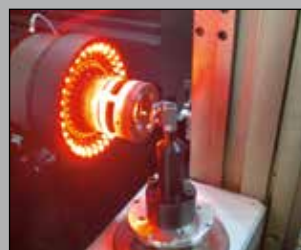
Measuring with multisensors: Calibration of the component using the Werth Fiber Probe 3D-WFP prior to measuring with the X-ray sensor.
