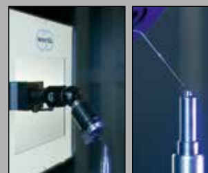
Measuring with multisensors: Diesel injectors: measurement setup with Werth Fiber Probe on the IP 40T sensor head.
