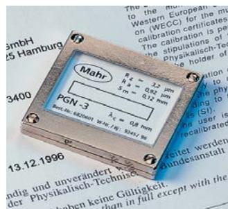
Surface standard with sinusoidal groove profile for dynamic monitoring of the roughness measuring station. Ra, Rz, Rmax.
