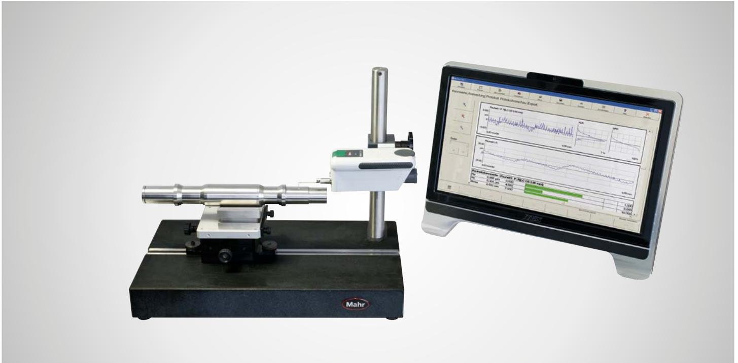
Measuring station for the measurement of roughness depths, P profile and waviness with the drive unit MarSurf SD 26 and the skidless probe system BFW 250.
