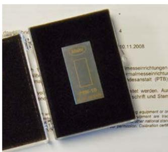
With Mahr calibration certificate. Roughness standard with turned profile, chromed. Profile depth ca. 10 µm (.394 µinch), for checking the roughness measuring station
