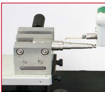
**Measurement of a stepped shaft**
