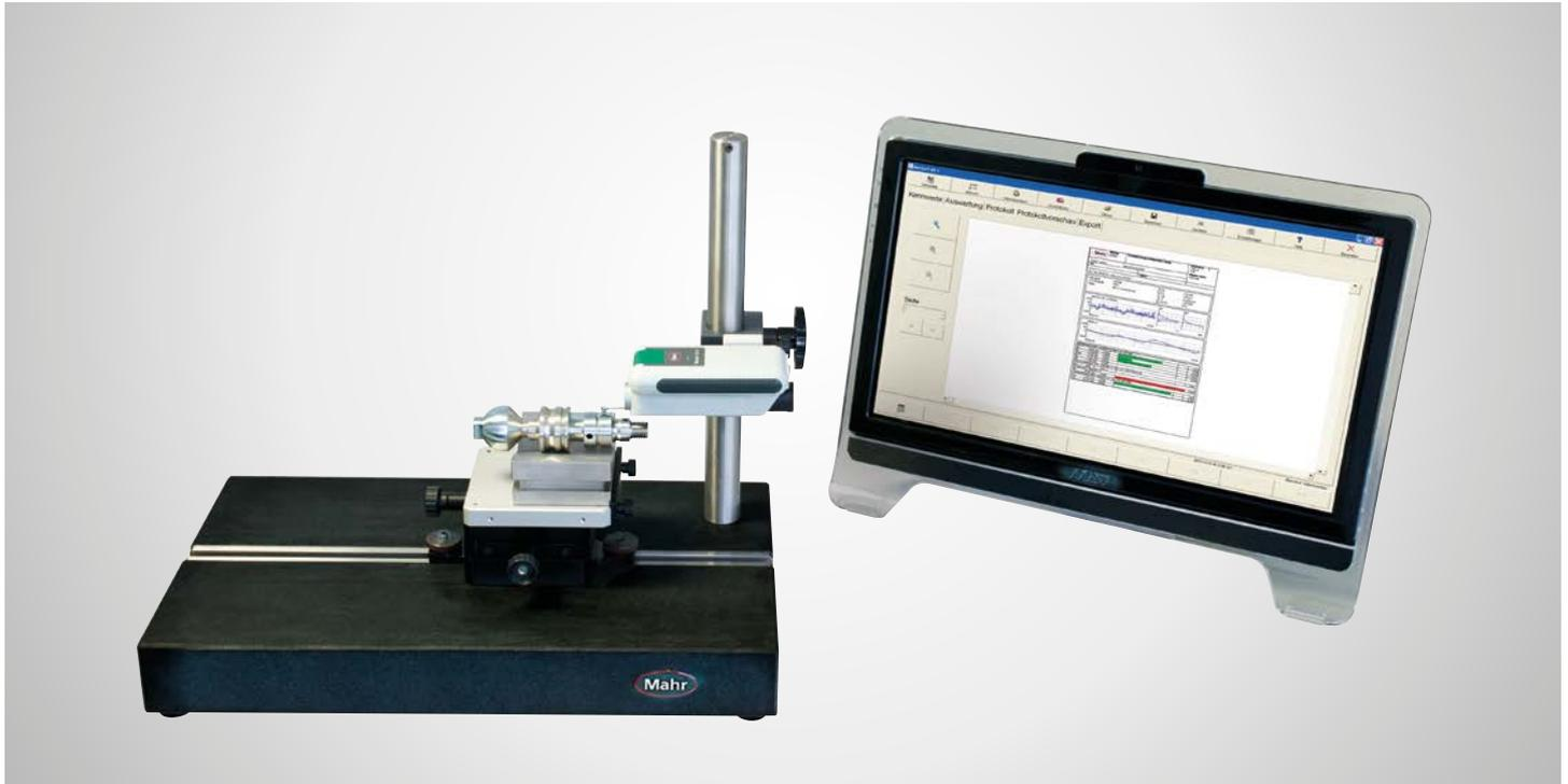
Measuring station for roughness measurements with drive unit MarSurf RD 18 and skidded probe PHT 6-350. This measuring station is characterized by easy and uncomplicated handling. All surface parameters based on roughness depth are available. The characteristics of the evaluation software
