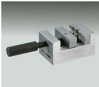
For mounting rectangular and cylindrical workpieces
