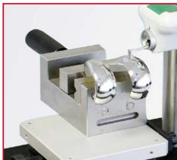
**Measurement of a knee joint**
