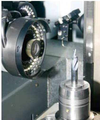
The basis for the high precision of Wolf's tools is the VideoCheck V HA multisensor coordinate measuring machine, which is equipped with WinWerth software.
