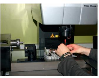
Figure 3. The measurement area was designed such that clamps and most fixtures can remain on the machine, which allows faster changeover of parts.
