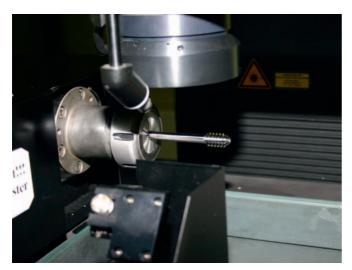
Figure 2. The additional fourth axis of the multisensor coordinate measuring machine simplifies measurement.
